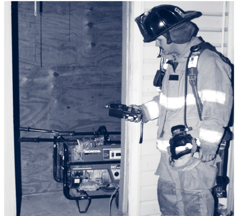
FIGURE 1. A firefighter uses a portable meter to measure the carbon monoxide (CO) level after CO exposure caused by a generator forced evacuation of an apartment building — Charlotte, North Carolina, 2003
